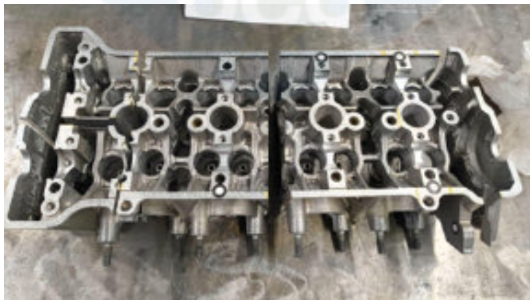
Figure 4: Sliced up engine head prepared for 3D scan and modeling. Credit: Yannis Leung
