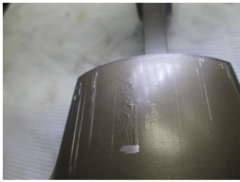
Examples of Ferroprint coating failures: early stages (left) & catastrophic (right)
