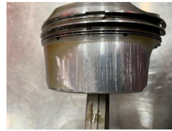
Examples of Ferroprint coating failures: early stages (left) & catastrophic (right)
